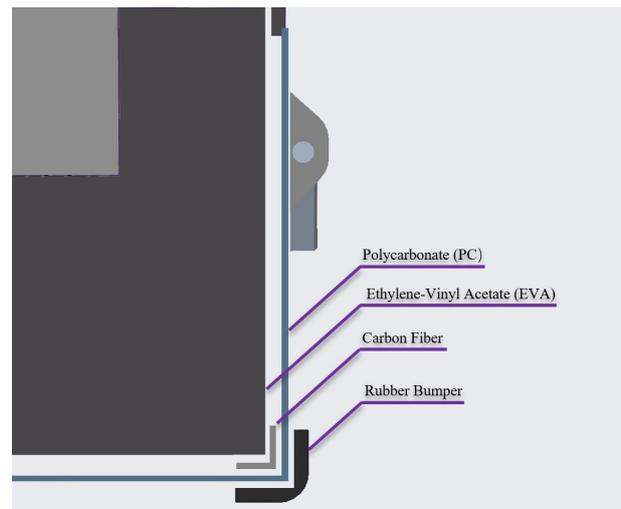
Figure 5. Multiple layers section view of the toolbox
